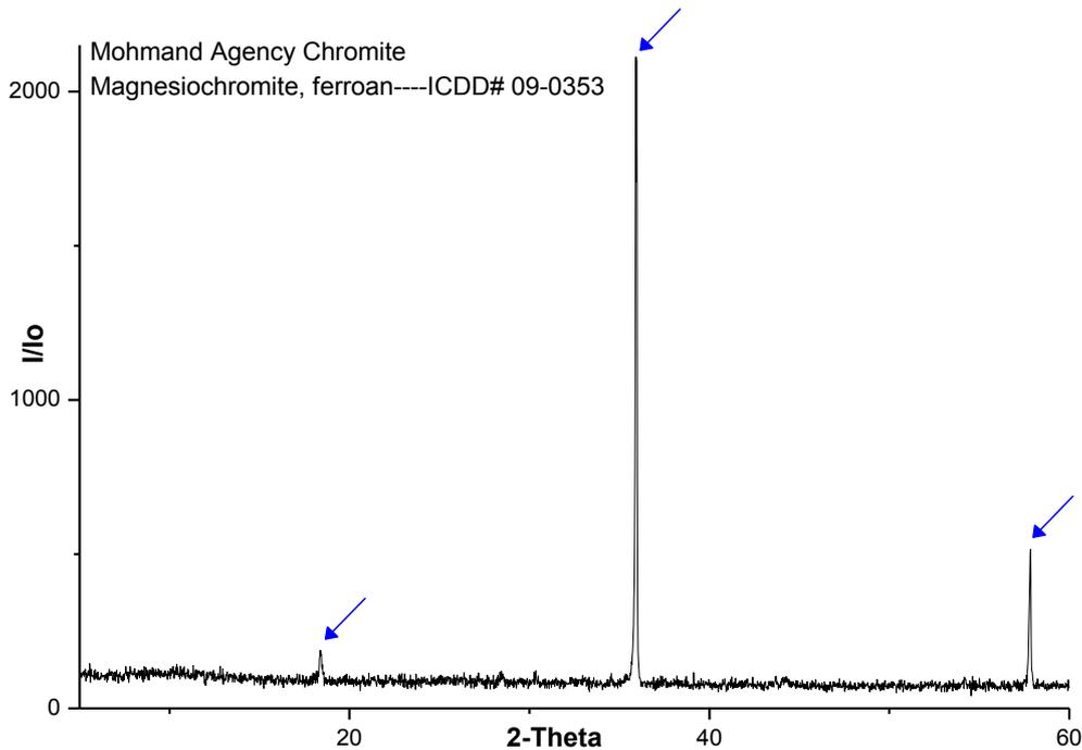
Figure 2. The XRD pattern of the Mohmand agency chromite, the data has possible match with ICDD card # 09-0353.
