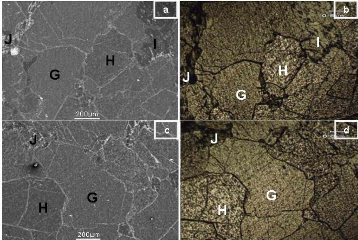
Figure 3. (a,c and (b,d) showing the SEI and MMI of the same regions respectively. EDX analysis suggested that the grains G and H represent chromite ore and I represent silicate impurities.
