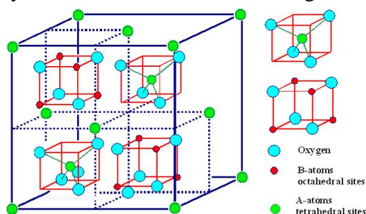
Figure 1. An  $\text{AB}_2\text{O}_4$  spinel structure<sup>1</sup>.
