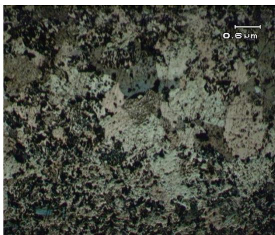
Figure 1a) Visual appearance of dolomite sample with ordinary camera and b) thin section photomicrograph of dolomite sample.
