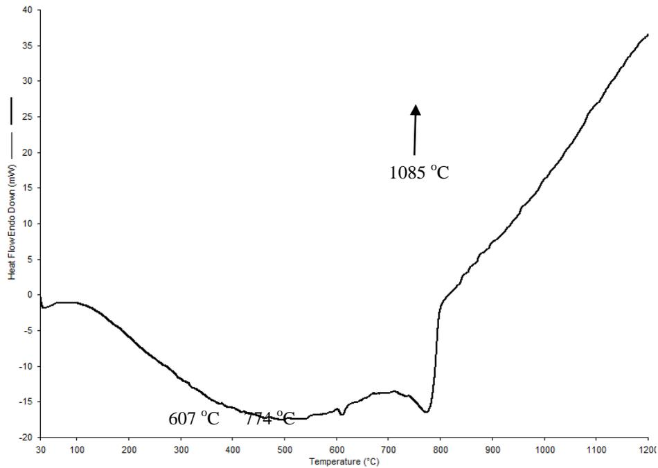
Figure 4. DTA pattern for dolomite sample, confirming the peaks observed in the DTG plot of the same sample.
