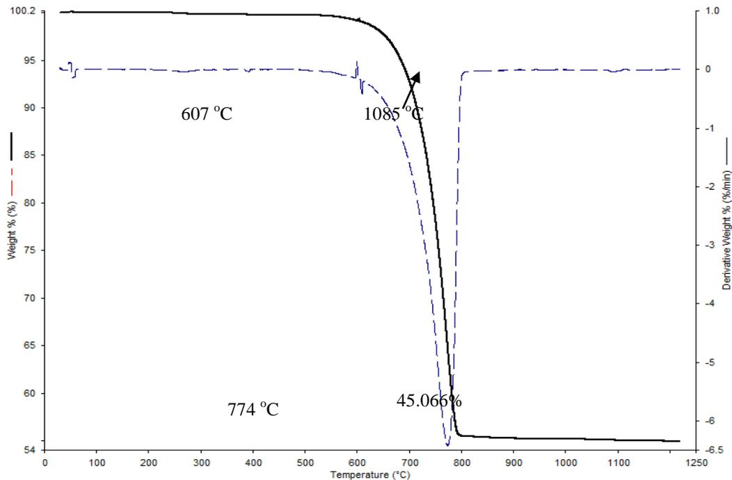
Figure 3. TG/DTG plot of dolomite sample collected a 10°C/min in N<sub>2</sub> atmosphere (at 20 ml/min) showing its thermal decomposition temperature.
