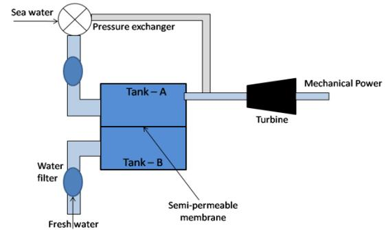
Figure 2. Schematic of an Osmotic power plant
